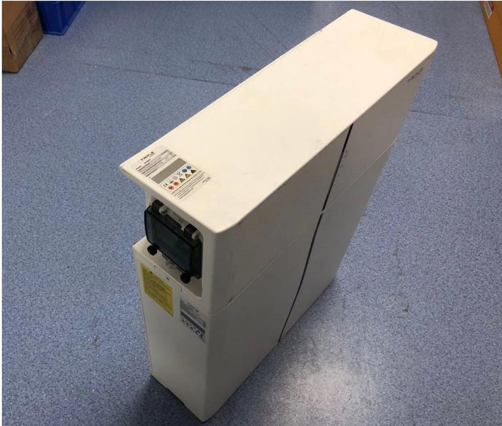
Picture 1 Photo of the battery module connected to the control box
