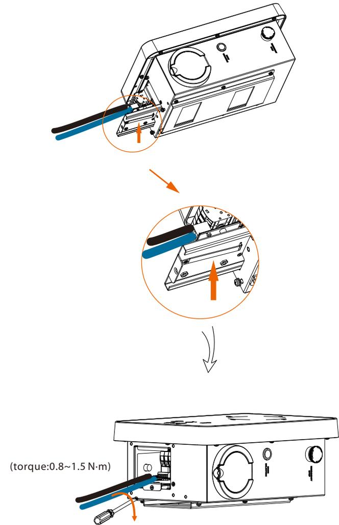
STEP 11: Push the rear cover to appropriate position of the cables and screw the self tapping screws with the cross screwdriver. Then tighten the waterproof fastening heads.
