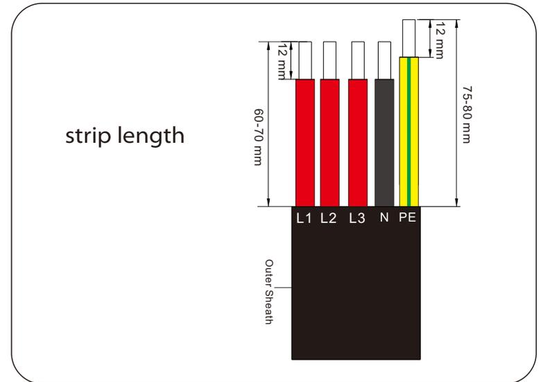
STEP 8: Insert the input cable through the waterproof connector in sequence as shown below.
